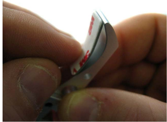
6. Position the rectangular tape pad on the inside of the second arm and press.
