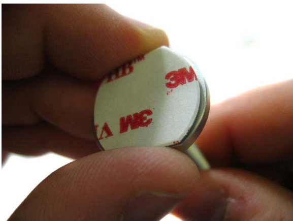
9. Ensure the straight edges and rounded edges line up. Press the tape against the disc.
