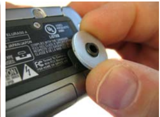
4. Place supplied washer on set screw.
