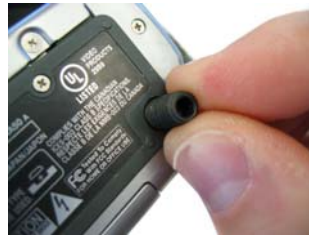
3. Ensure that Allen hole is facing you.
