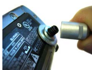
7. Thread security nut onto set screw.
