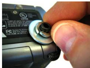
5. Place supplied lock washer on set screw.
