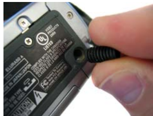
2. Thread set screw into tripod mount.
