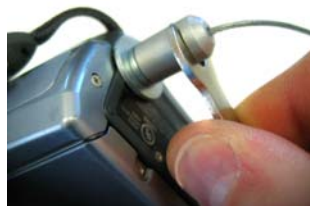
9. Tighten gently with security wrench.
