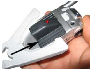
6. Slide Removal tool [120100] under sensor and break tape bond.
