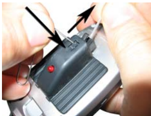
5. Insert paperclip, press down and pull cable.
