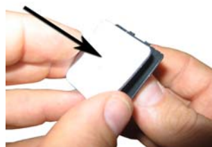
7. Remove old tape and apply a new tape pad [120100].
